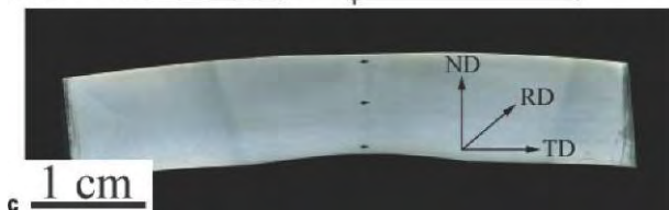
a orientation of as welded sample relative to steel processing directions: top and bottom line is near outer and inner surfaces of pipe respectively, while middle line is in mid-thickness of pipe, b orientation of Charpy specimen and c joint segment after post-welding heat treatment
