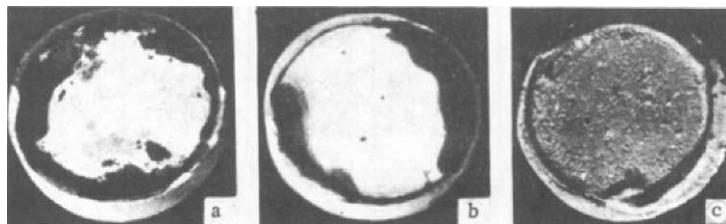
Fig. 2. Supports of zirconium—hafnium solid solutions (a, b) and zirconium dioxide (c) after heating to 2300°C with molybdenum billet.
